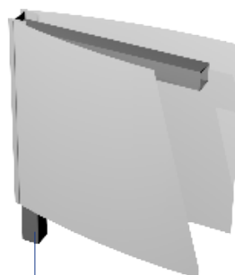
Aluminium or steel profile 60 x 60 x 4mm Tube de fondation 60 x 60 x 4mm
